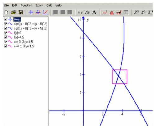
From the graphs we see that the system has one root, which is within the square  $[3, 4.5] \times [3, 4.5]$  (the red square at the above picture). We use the computer program to find the root of the function f(x,y) = |f1| + |f2|, where f1 and f2 are the left sides of the equations of the system. Set N = 15. We require 10 true digits after the decimal point. The answer is as follows: x = 3.6195014038, y = 3.8284457768, so that we obtain r = 2.0344577679.
